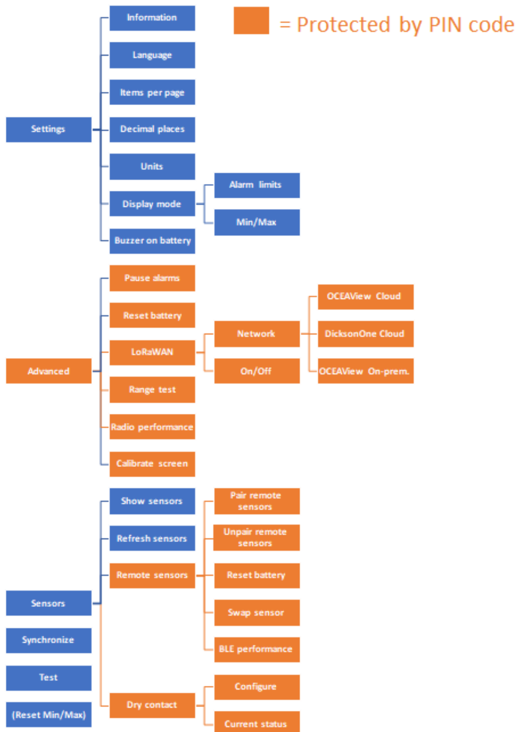
Figure 28 – Menu structure when using LoRaWAN wireless operation
