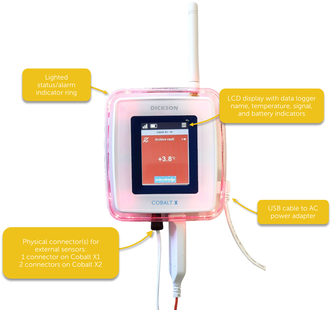
Figure 4 – Cobalt X2 data logger with two external sensors
