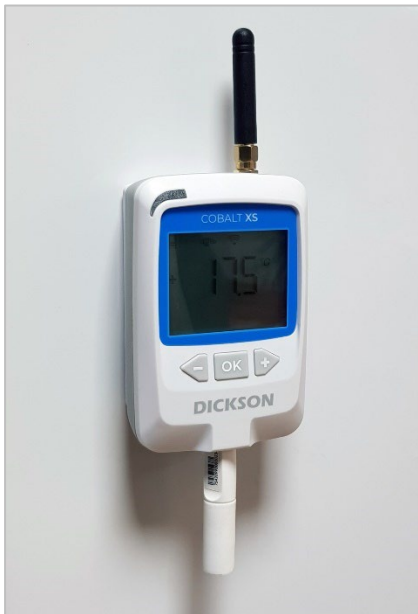
Figure 11 – Mounting the Cobalt XS on a metallic surface with magnets
