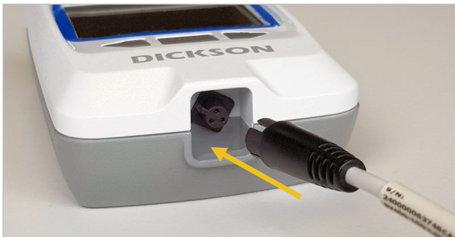
Figure 13 – Plugging a sensor into the Cobalt XS data logger
