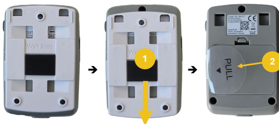
Figure 1 – Remove the cradle and pull out the plastic tab to activate batteries
