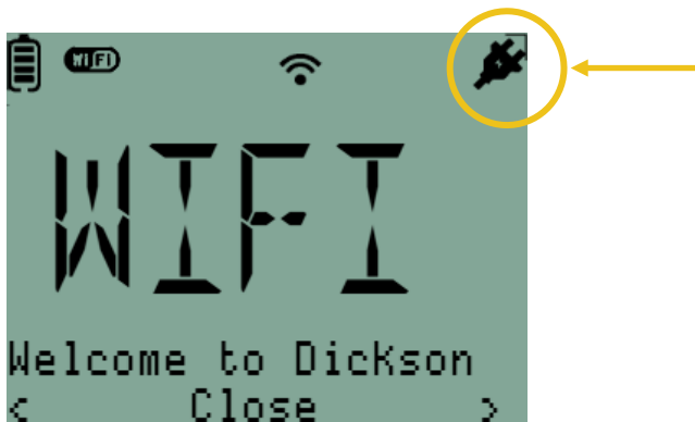
Figure 13 – Data logger plugged into external power source
