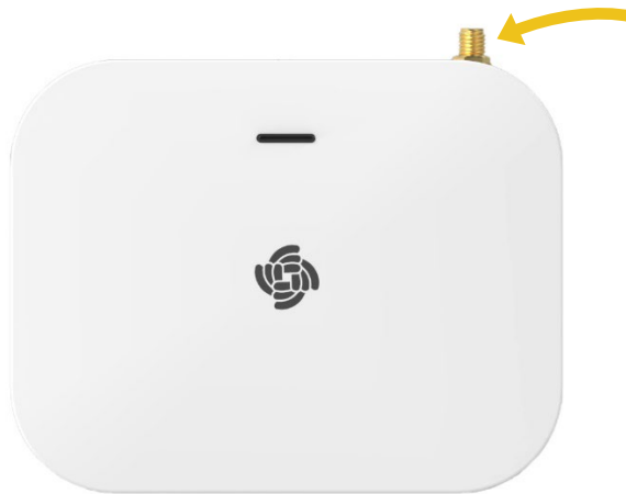
Figure 3 – Attach LoRaWAN antenna to connector
